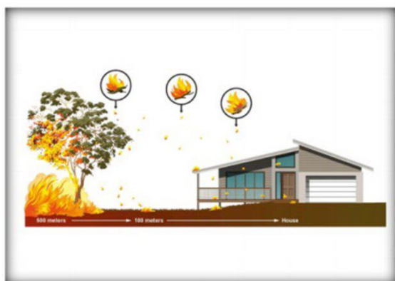
Figure 6 Ember attack on structure
