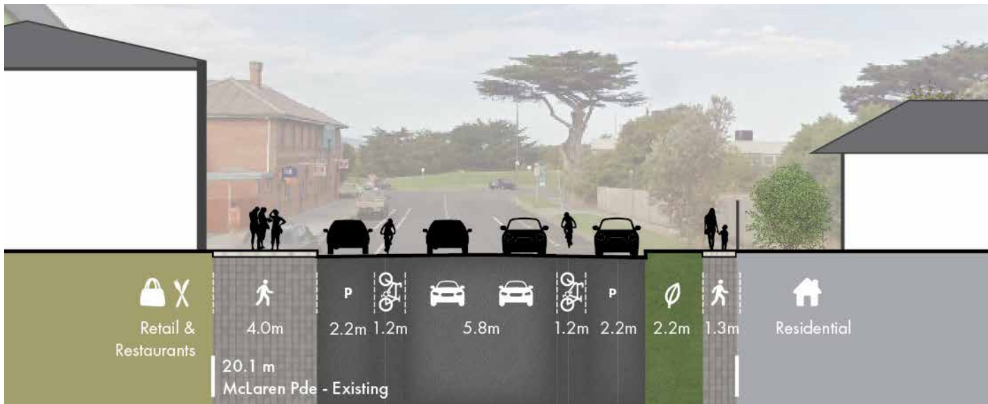
Figure 41. McLaren Parade A-A' - Existing Cross Section
