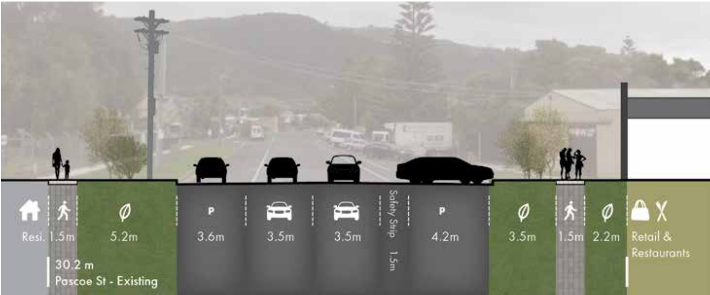
Figure 25. Pascoe Street B-B' (Between Hardy St And Moore St) - Existing Cross Section PLEASE NOTE: Dimensions indicative only and based off Nearmap Aerial.
