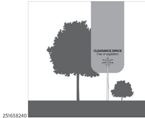
GRAPH 6 - MINIMUM CLEARANCE SPACES SURROUNDING A POWERLINE— UNINSULATED 66kV ELECTRIC LINE in HAZARDOUS BUSHFIRE RISK AREA
