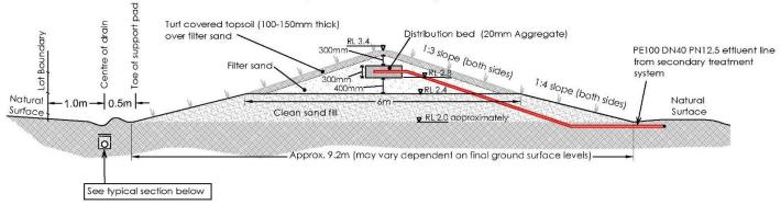
The design for the WWTP must satisfy all current and applicable codes of practice under the Environment Protection Act (EPA Publication 891.4) and Australian Standards (AS 1547:2012). Based on the expected toilet demand, the mound will receive a maximum of 3,000 Litres/per day of UV treated wastewater.
