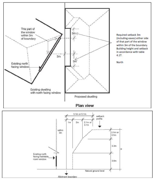
**Regulation 82(2)** - This regulation defines the orientation of a north facing window The diagram below shows the orientation from north of a "north facing window".
