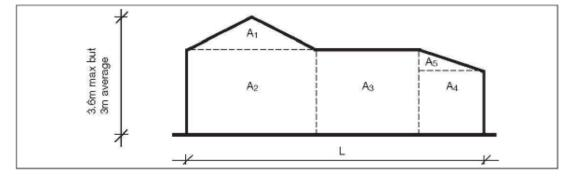
**Regulation 80(4) Height of Wall Or Carport On Boundary -** The average wall height (HA) can be calculated as follows: HA = A1 + A2 + A3 + A4 + A5 L where A1 A2 A3 A4 A5 equals the area of that part of the wall.
