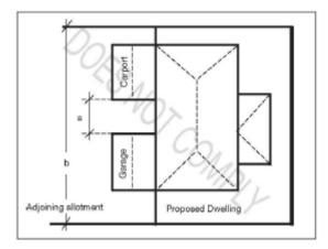
**Regulation 80(3)(B) Walls On Boundaries -** The diagram below shows how regulation 80 relates to that part of the subject boundary as it interfaces with each adjoining allotment
