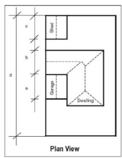
Regulation 80(3)(A) Length Of Walls On Boundary - THE PROPOSAL SHOWN BELOW DOES NOT COMPLY The portion of the proposed wall marked (a) is not abutting an existing wall or a carport on an adjoining allotment and the length of the proposed wall is also greater than 10m plus 25% of the remainder of the length of the boundary (b). The proposal requires a consent from the relevant council.
