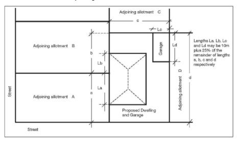
**Regulation 80(4)** – **Height of walls on boundaries** - The average height of a wall on a boundary is not to exceed 3m. The average height is calculated by dividing the total area of the wall by the total length of the wall.
