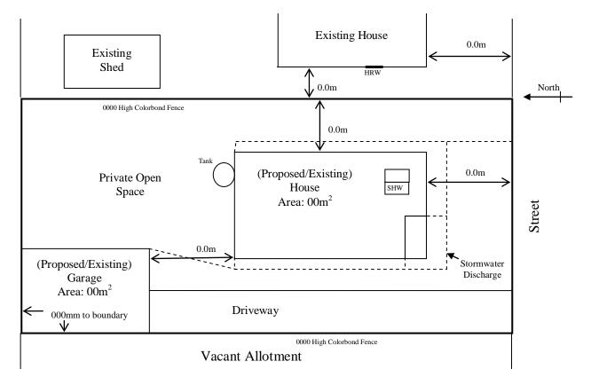
**Floor Plan** – Birds eye view of proposed works, including existing works, proposed works, room use, amenities, and dimensions (including doors & windows)
