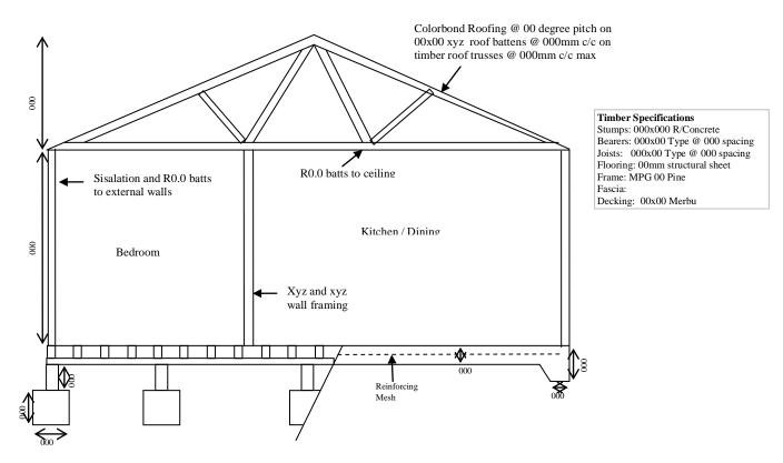
**Elevation** – View of building works from each direction showing features, heights, articulation joints, sub-floor ventilation, and materials used
