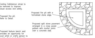
PROPOSED FIRE PIT Detail Plan - Scale 1:50
