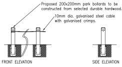
PROPOSED BOLLARD DETAIL Elevation - Scale 1:50
