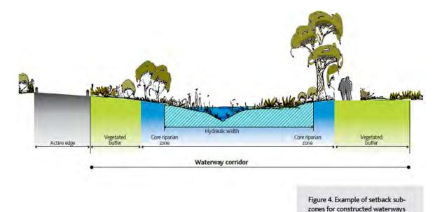
Figure 8.2 Constructed waterway corridor typical cross section
