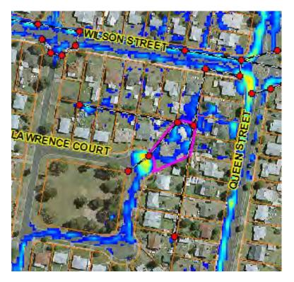
Figure 6.8 Flooding at 11 Lawrence Street as predicted by flood model (5 year ARI)
