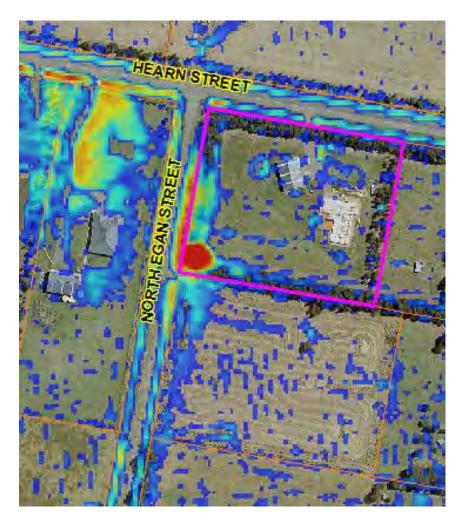
Figure 6.6 Flooding at 18 Hearn Street as predicted by flood model (10 year ARI)
