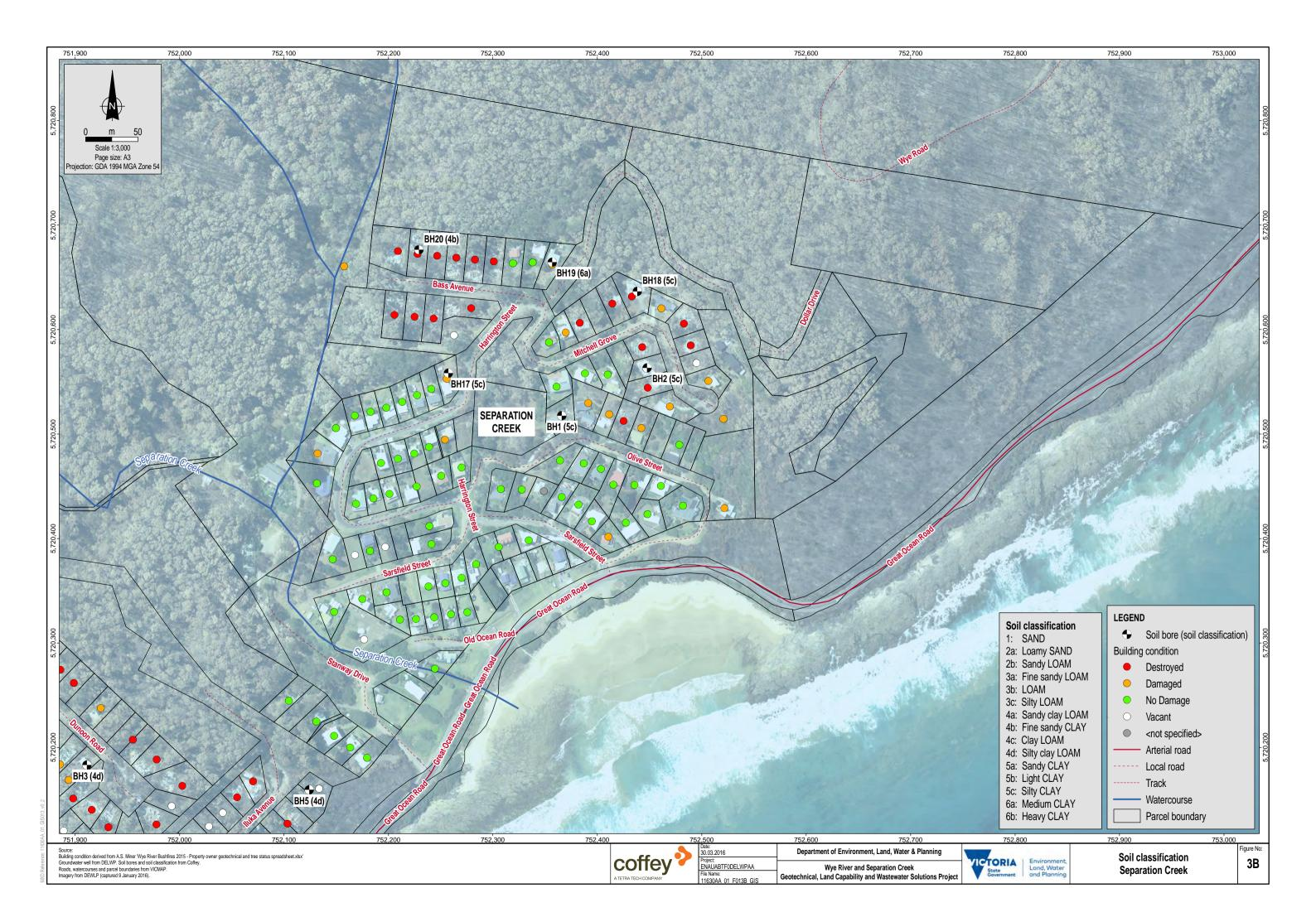
The soil profile at Separation Creek was found to typically comprise brown silty clay with moderate structure (Figure 3b). The depth to rock also varies but is typically intersected at approximately 1 metre below ground surface (mbgs). The indicated permeability (Ksat) of these shallow soils is likely to range between 0.06 to 0.12 m/day.
