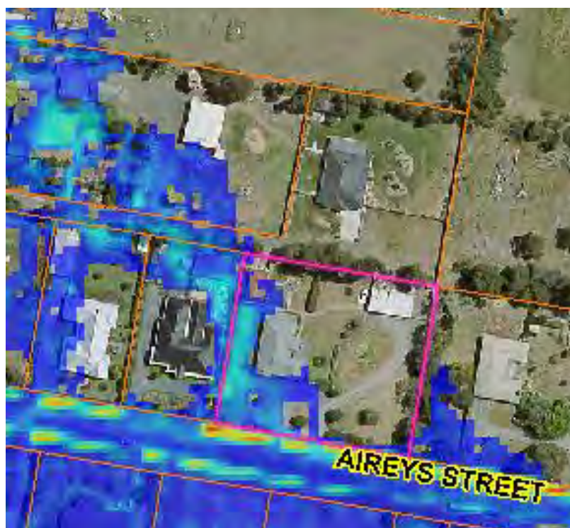
Figure 6.10 Flooding at 177 Aireys Street as predicted by flood model (10 year ARI)
