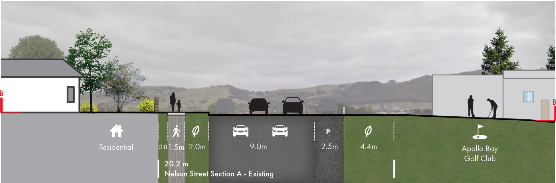
Figure 32. Cross Section B-B' - Nelson Street - Existing Conditions
