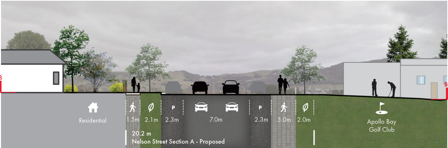
Figure 34. Cross Section B-B' - Nelson Street - Proposed
