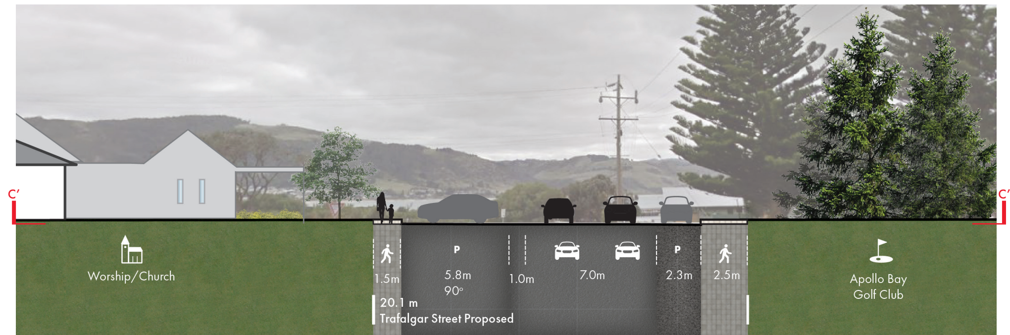
Figure 38. Cross Section C-C' - Trafalgar Street - Proposed
