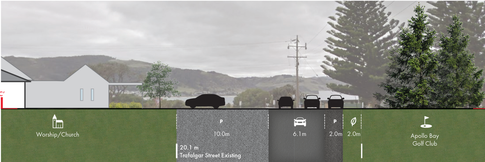
Figure 36. Cross Section C-C' - Trafalgar Street - Existing Conditions
