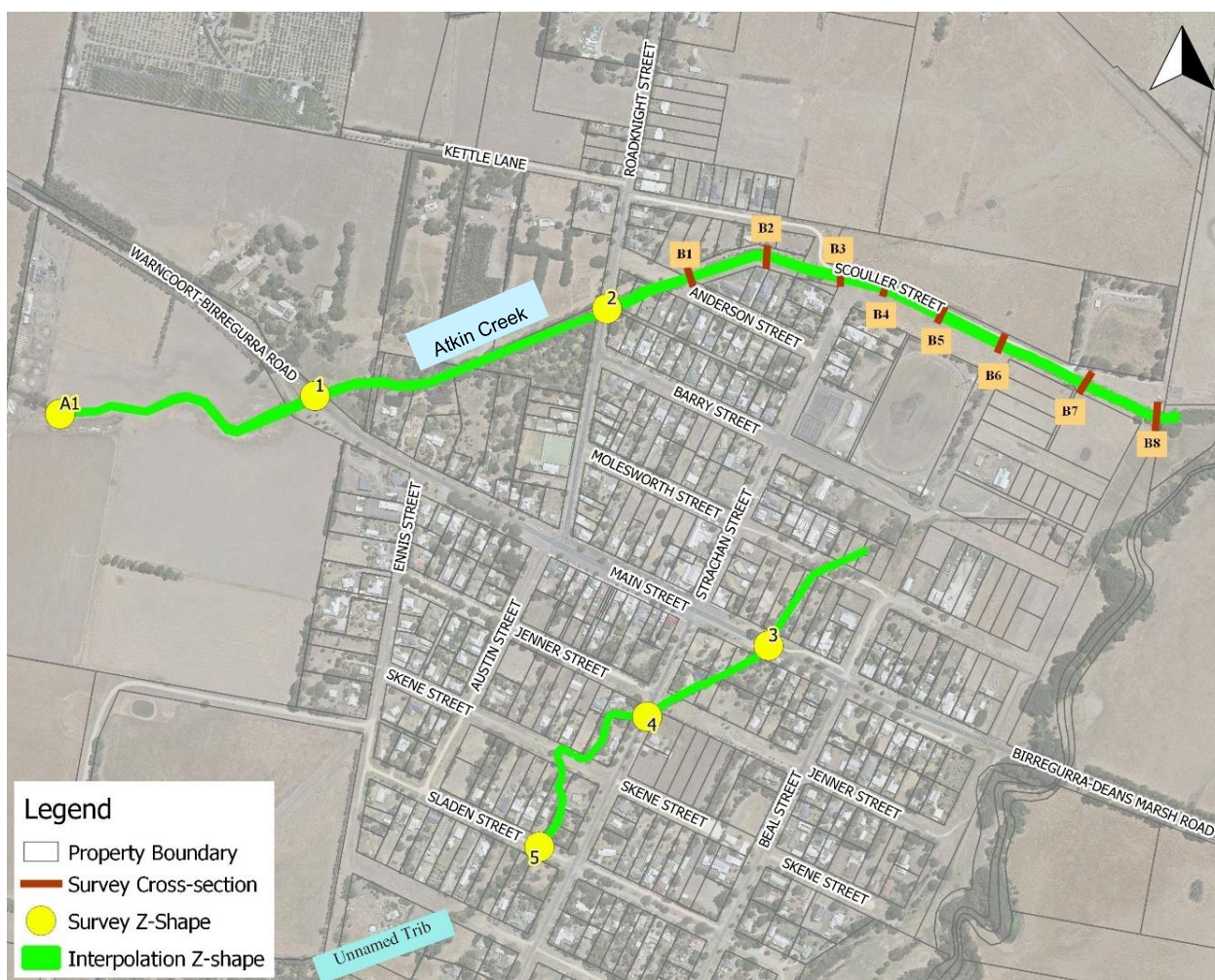
Figure 4.2: Location of Model's Terrain Modifications Informed by Survey Cross-Sections
