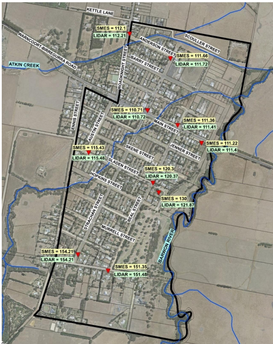
Figure 2.2: LiDAR Verification to Known Survey Marks
