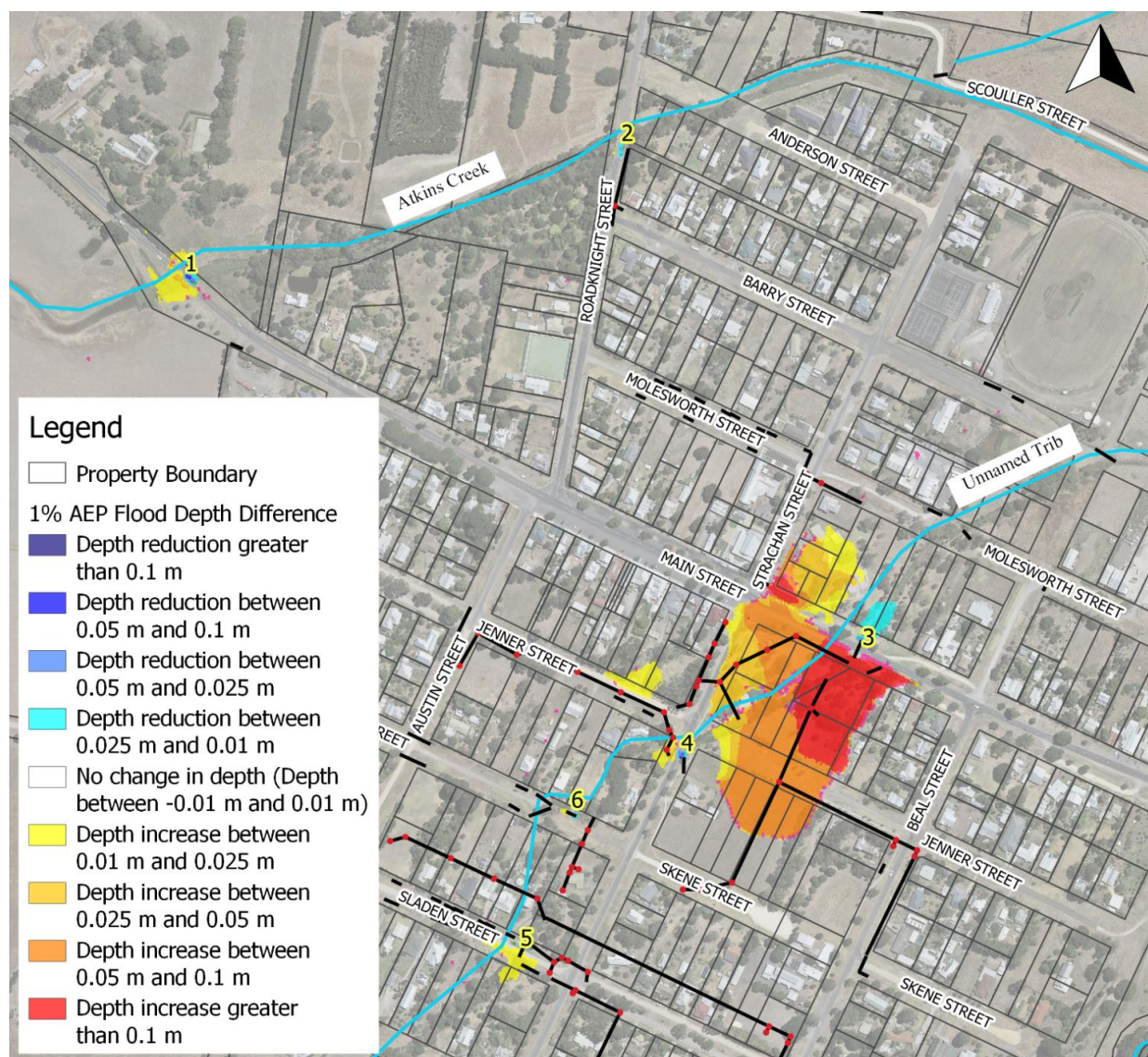
Figure 4.13: 1 % AEP Blockage Sensitivity Scenario Flood Depth Difference
