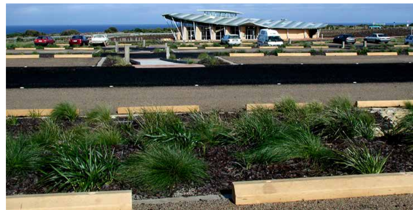
Image 61. Potential for passive irrigation of plants within car park area (i.e. utilising stormwater runoff).
