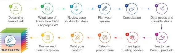
The Step by Step Guidance section of FLARE highlights important considerations for the initial planning and decision making of setting up a flash flood warning system (Flash Flood WS).
