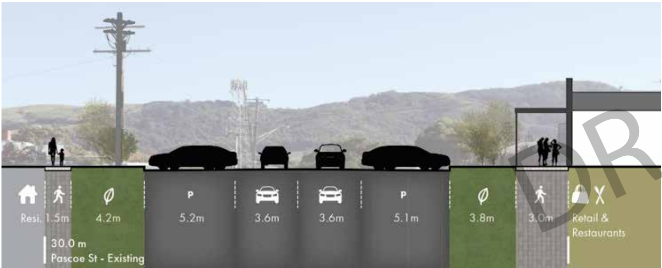
Figure 30. Pascoe Street A-A' (Between Moore St And Nelson St) - Existing Cross Section PLEASE NOTE: Dimensions indicative only and based off Nearmap Aerial.
