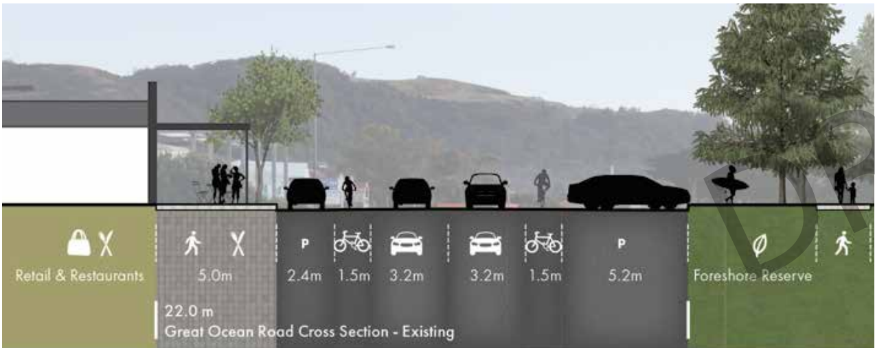
Figure 26. Great Ocean Road A-A' - Existing Cross Section
