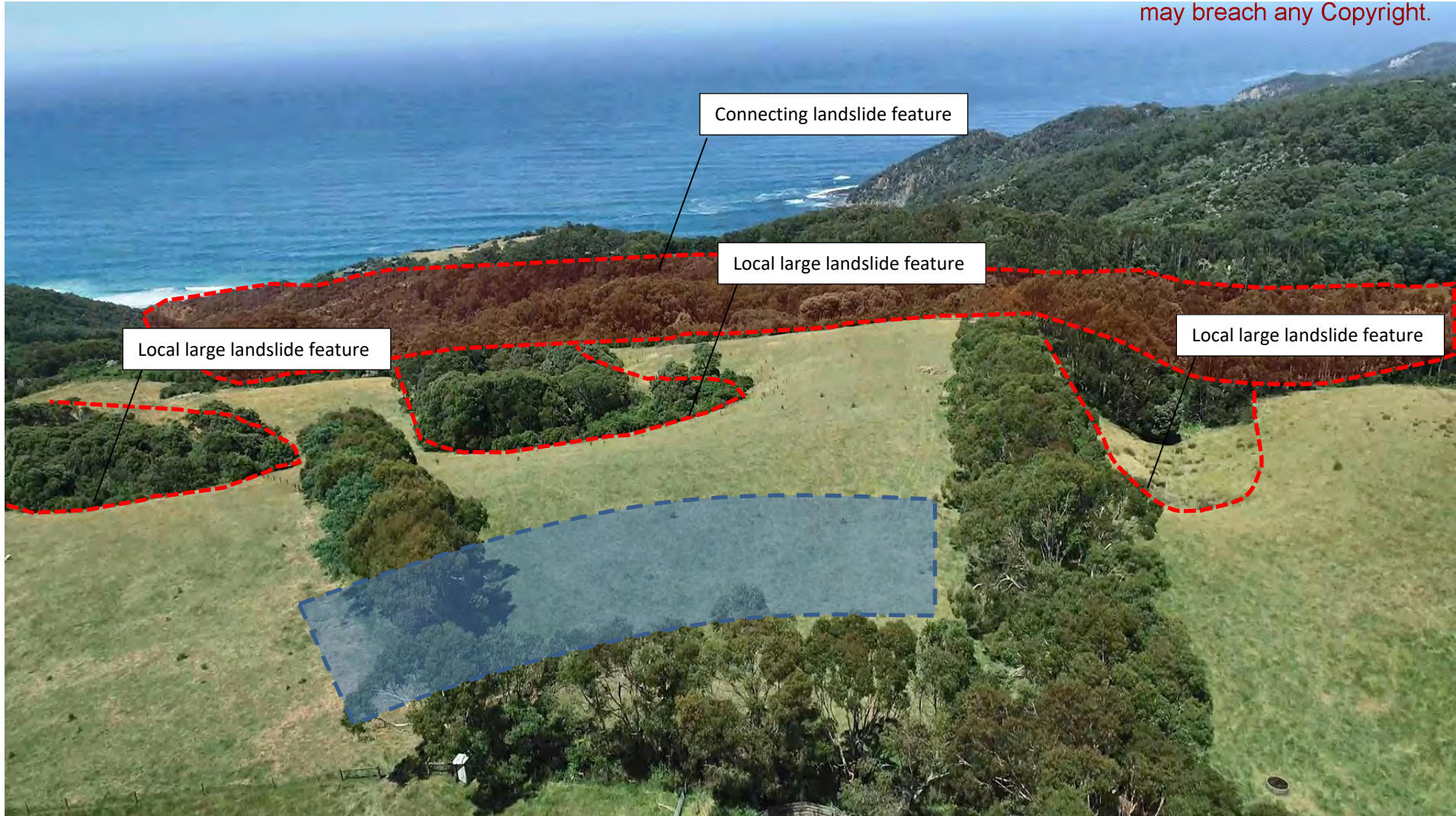
Aerial photograph of proposed dorm development area and inferred landslide
