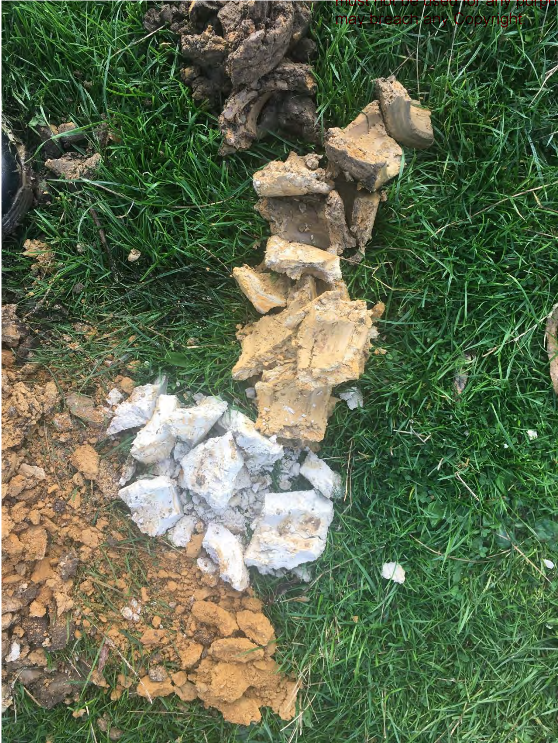
Typical soil/rock profile, (borehole 3)
