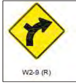
Figure 5.1: Signage for side road intersection on outside of curve
