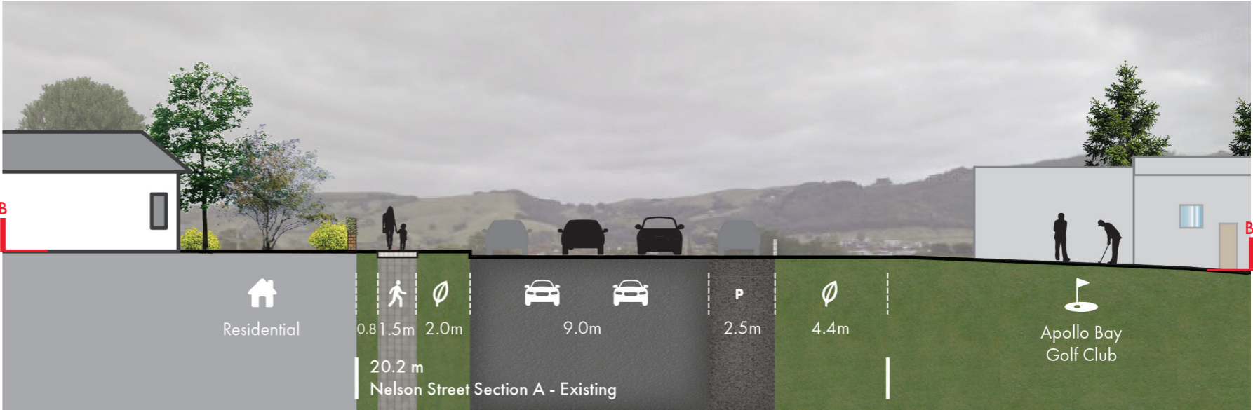
Figure 31. Cross Section B-B' - Nelson Street - Existing Conditions
