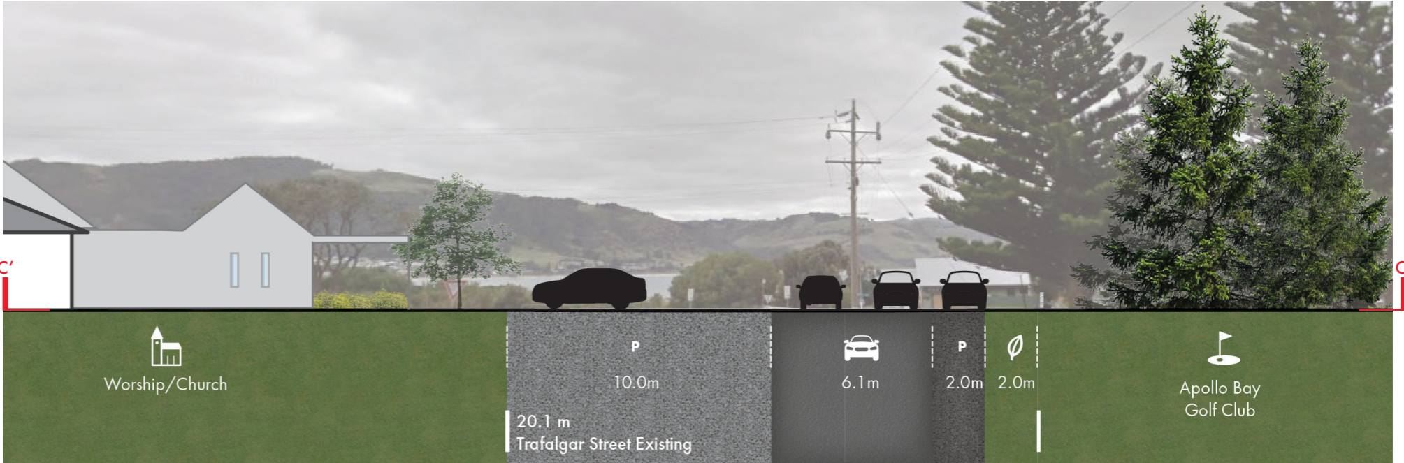
Figure 35. Cross Section C-C' - Trafalgar Street - Existing Conditions
