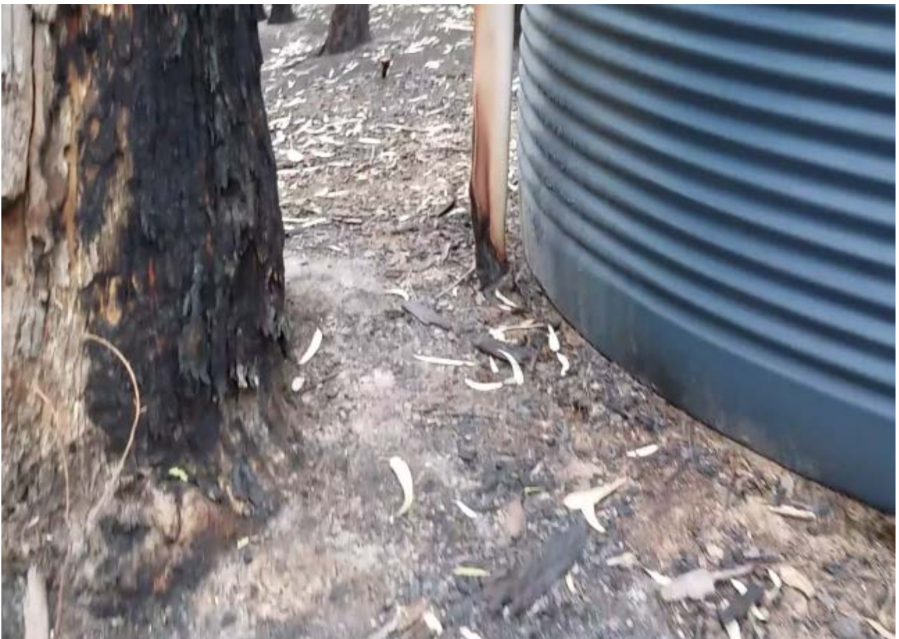
Figure 70: Some fire interaction between a burning tree trunk and an adjacent polyethylene water tank. The ground surface and tree bark condition indicate the suppression had occurred in this area.
