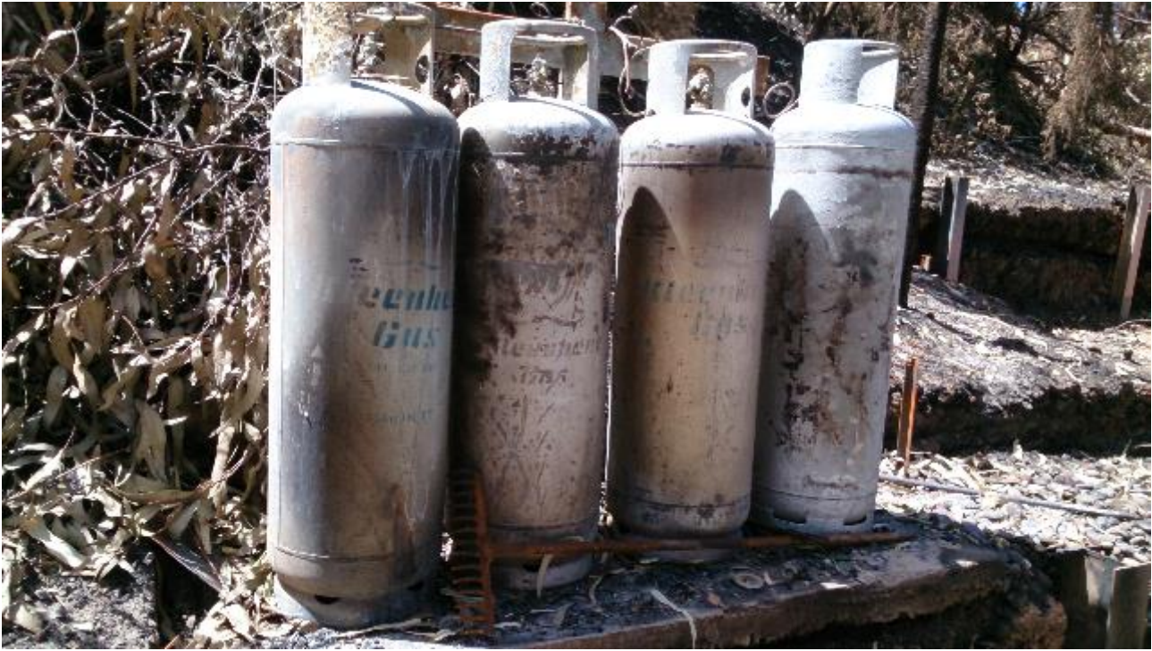
Figure 51: LPG pressure vessels adjacent to house.
