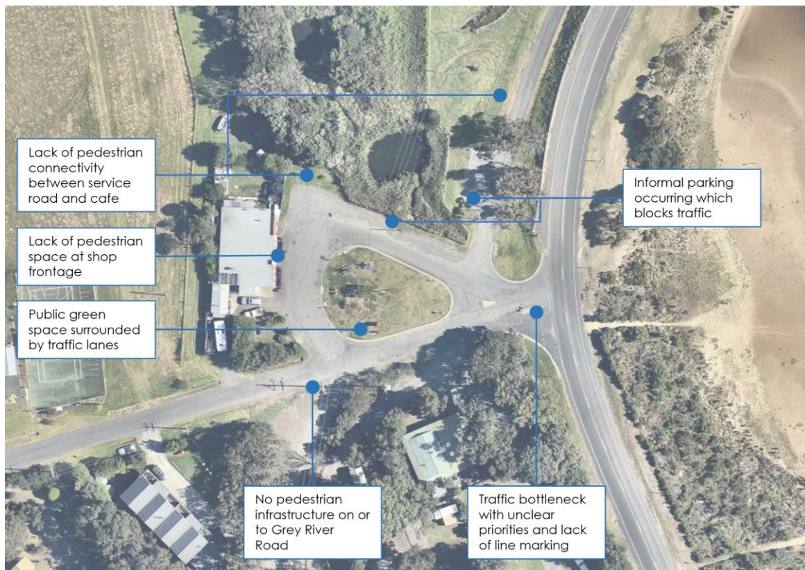
Figure 5.2: Issues Identified with the Roundabout at the Entrance to Kennett River
