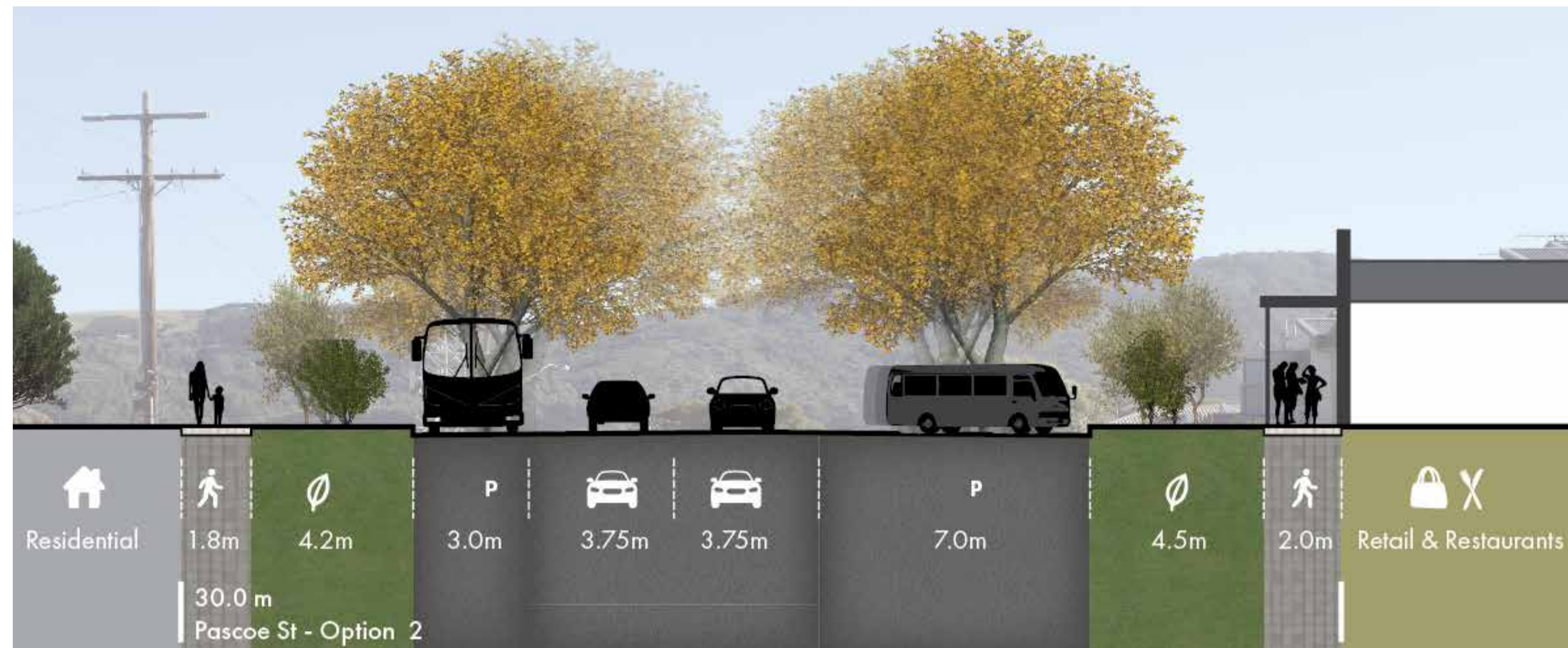
Cross Section - On Street Bus Parking
