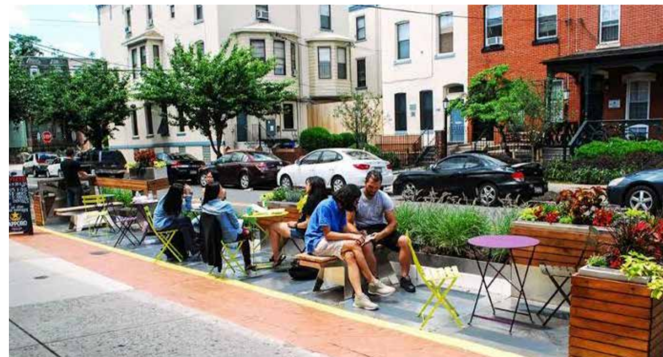
C.8 Planter boxes and temporary kerbs used to delineate expanded footpath.
