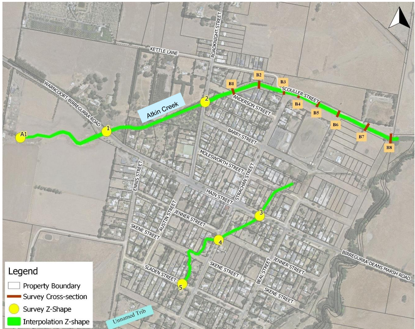
Figure 4.2: Location of Model's Terrain Modifications Informed by Survey Cross-Sections
