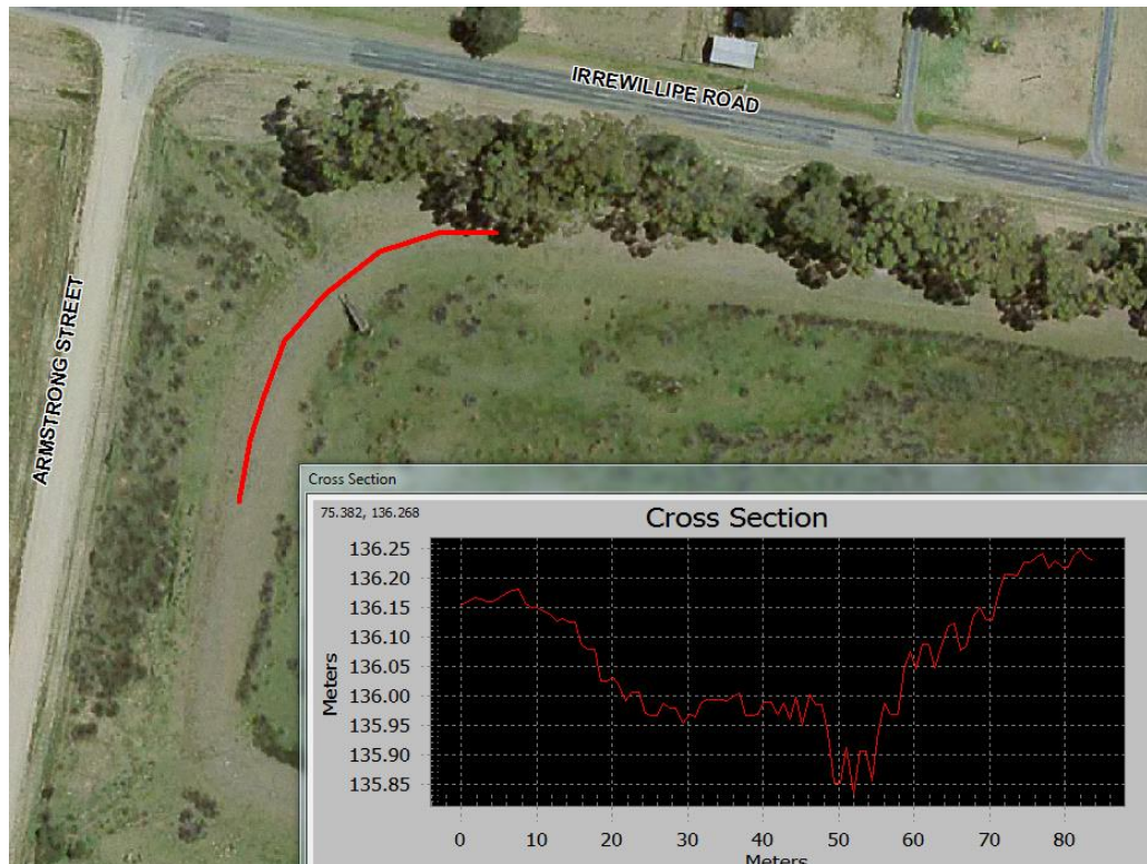
Figure 3.3 Existing embankment spillway profile
