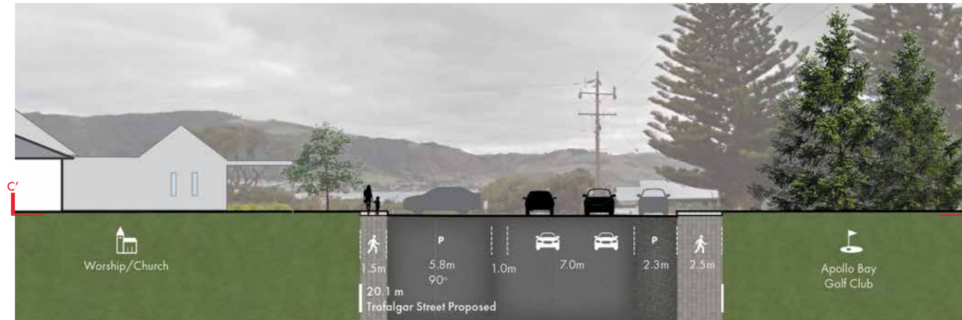
Figure 37. Cross Section C-C' - Trafalgar Street - Proposed
