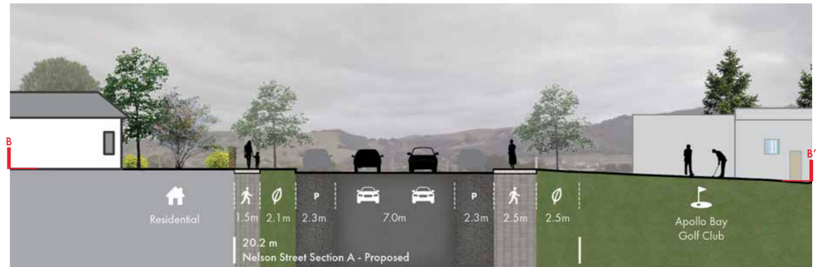
Figure 33. Cross Section B-B' - Nelson Street - Proposed
