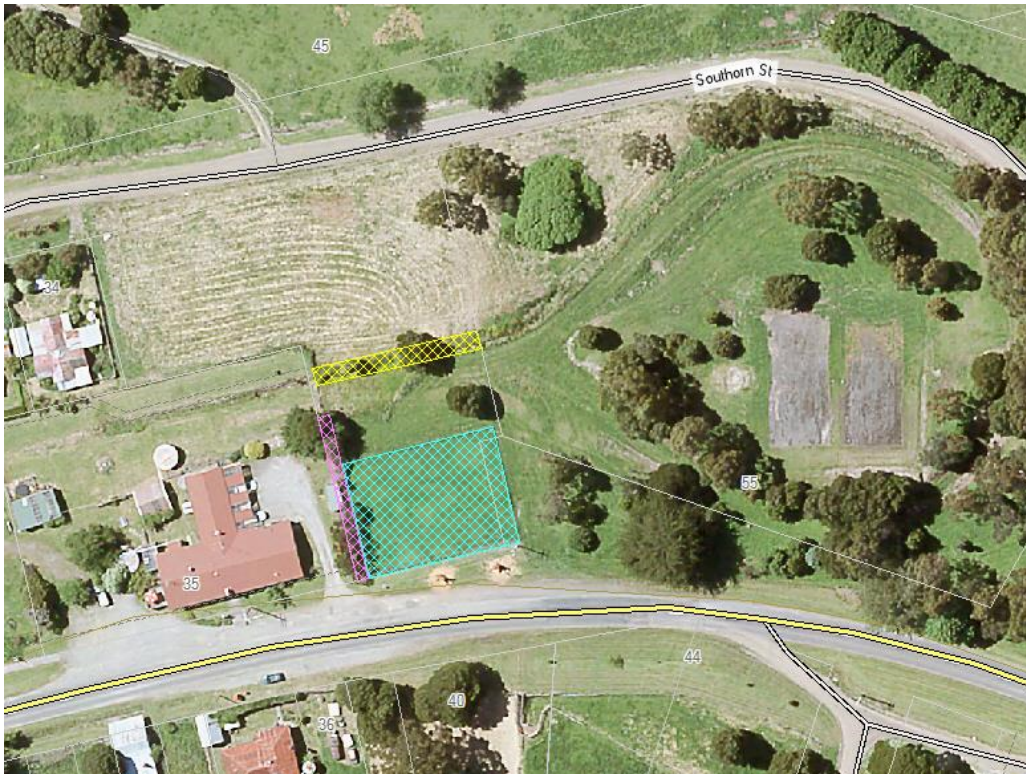
Figure showing location of gravelled area (green), steel fence (pink) & earth mound (yellow).
