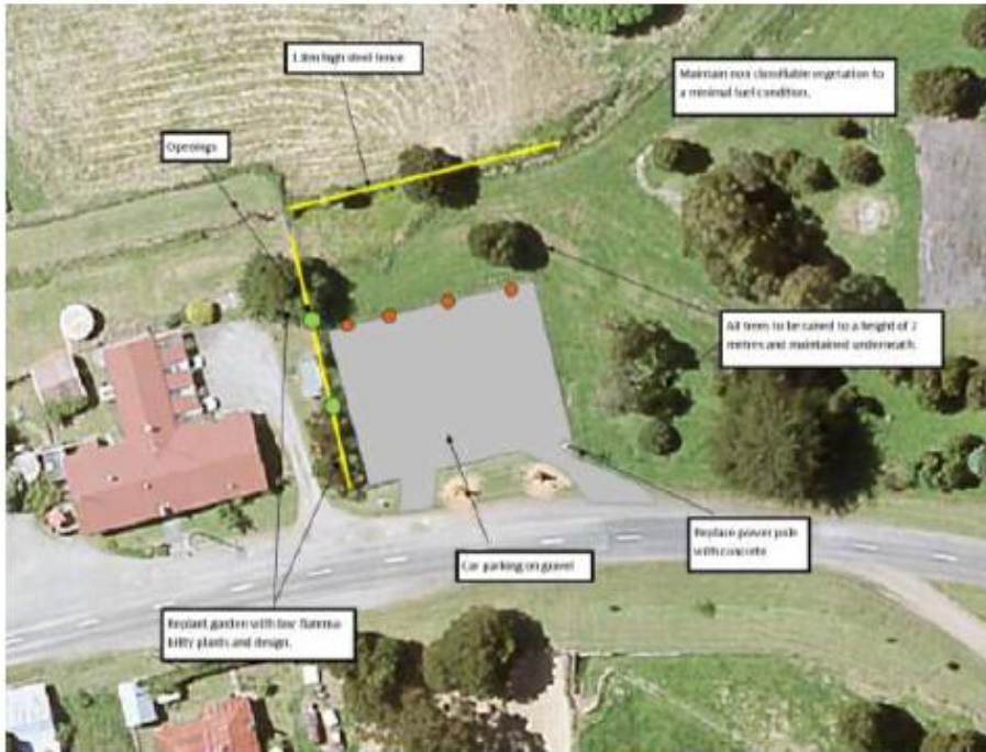
Figure 12. Proposed site design to achieve further radiant heat attenuation and safety
