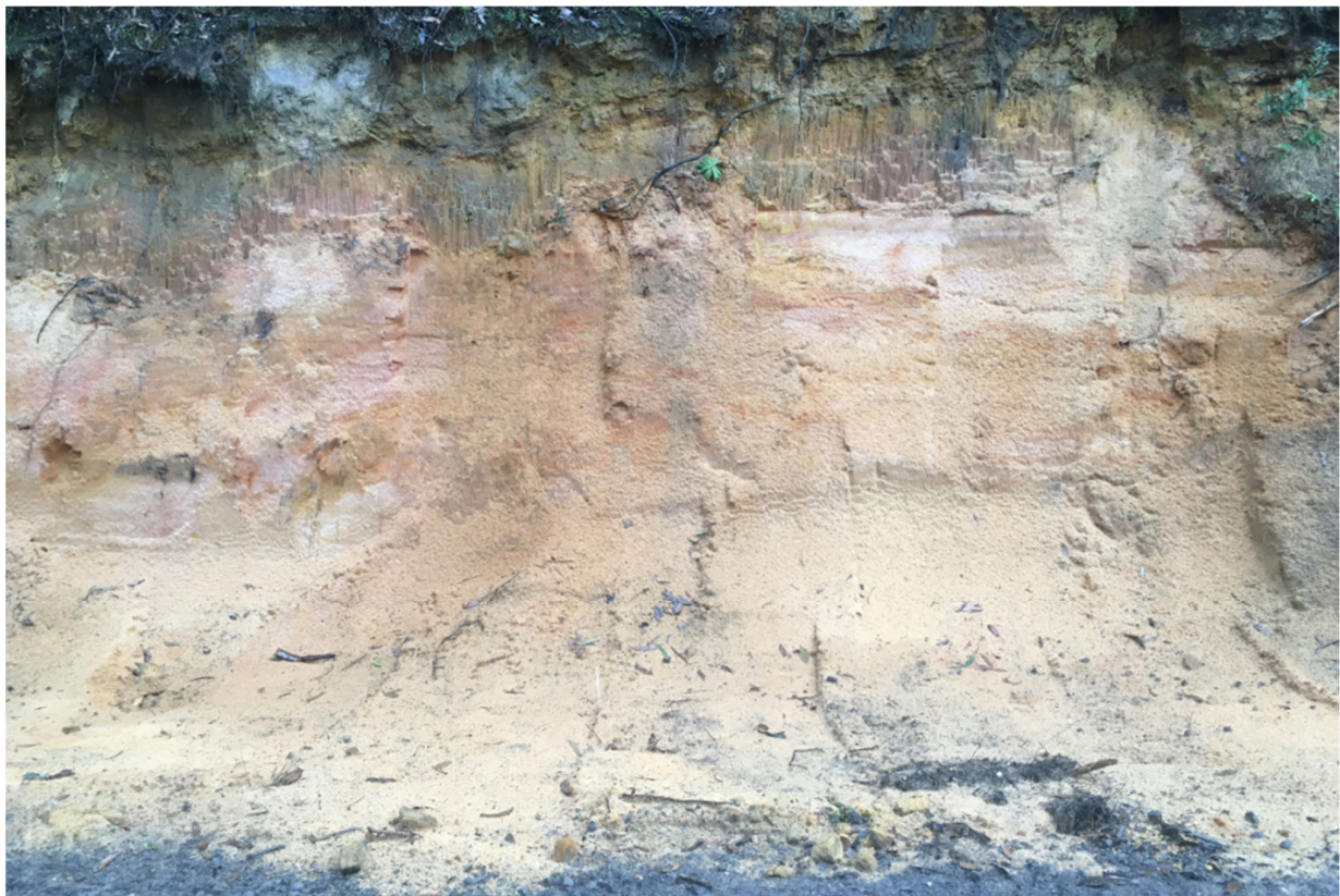
Photo 11: Sand (inferred Pwe, but close to the geological boundary with Pwm) exposed in a road cutting on the Gellibrand-Carlisle River Road.
