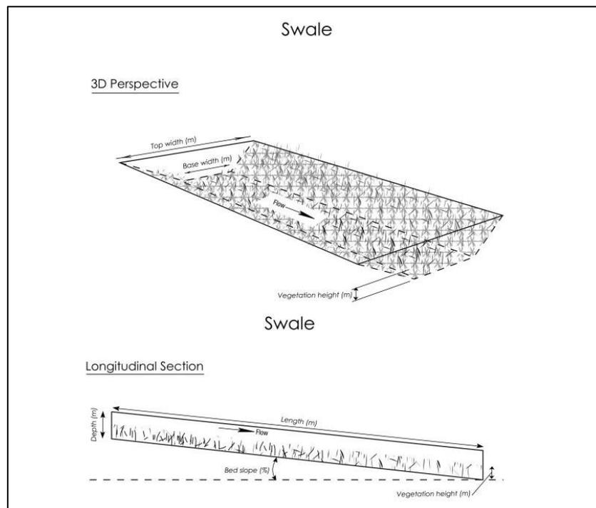
Figure 4-6 Conceptual diagram of swale properties
