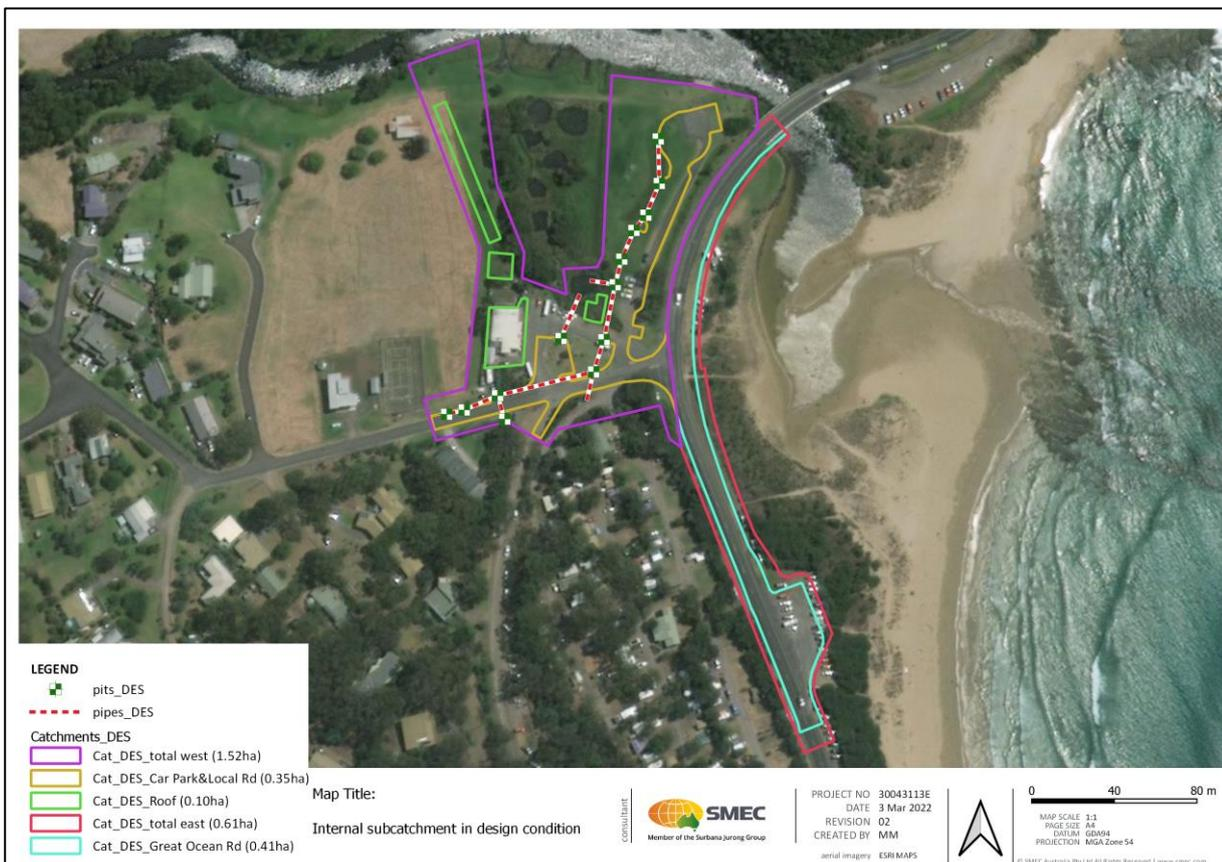
Figure 3-4 Internal subcatchment in design condition
