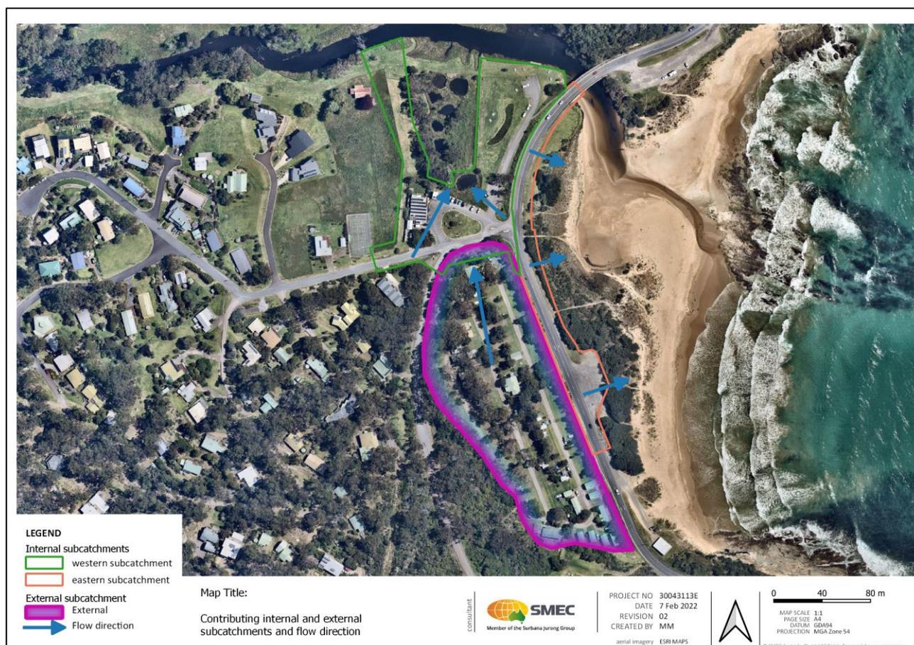
Figure 3-1 Contributing internal and external sub-catchments and flow direction
