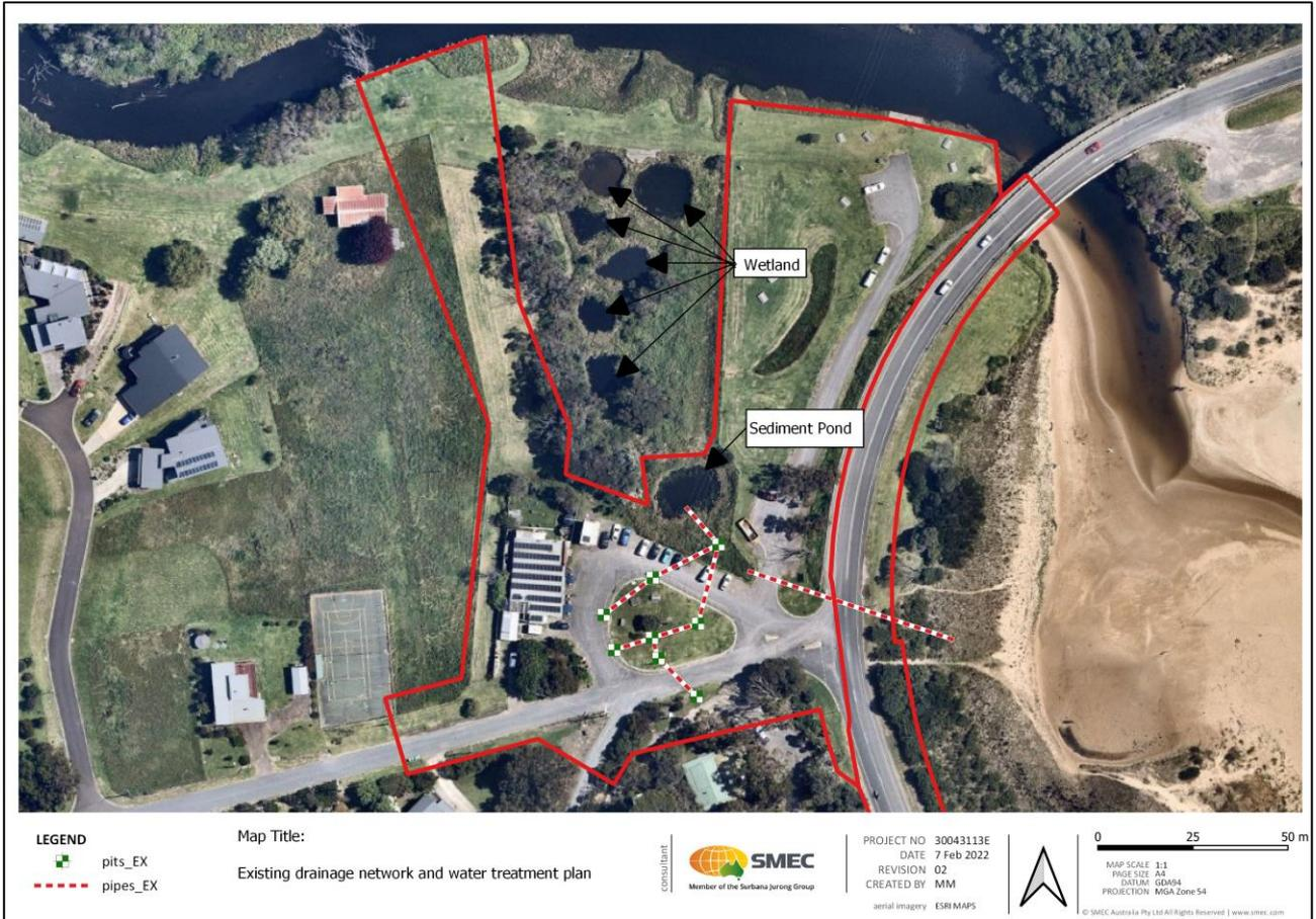
Figure 2-2 Existing Pits and Pipes network and water treatment plant including sediment pond and wetland
