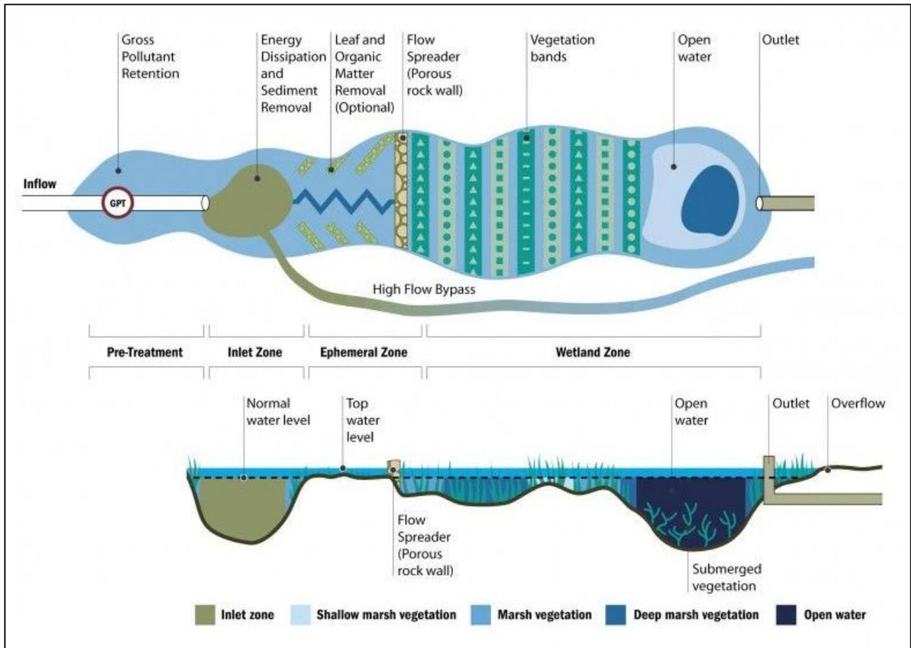
Figure 4-2 Schematic representation of a typical wetland (adopted from [www.urbangreenbluegrids.com](http://www.urbangreenbluegrids.com))
