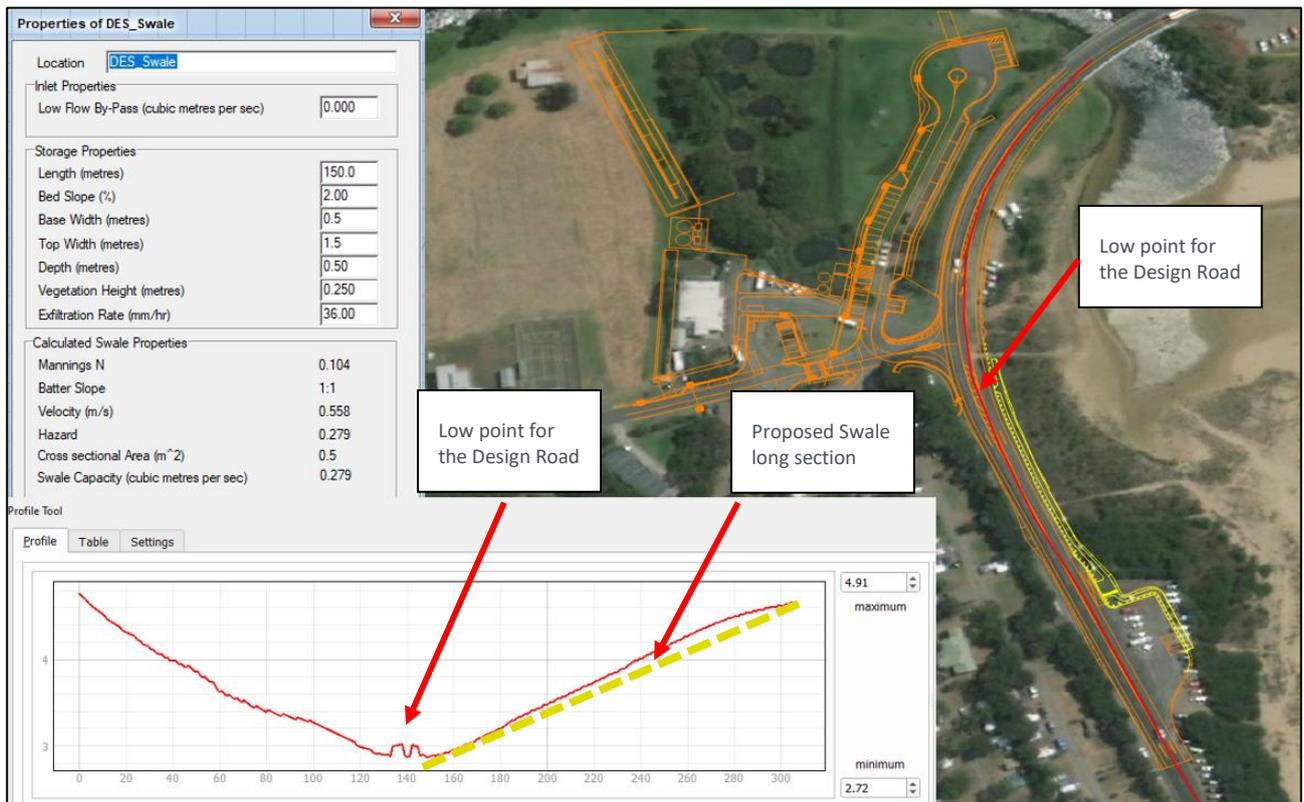
Figure 4-7 Proposed swale location and specification
