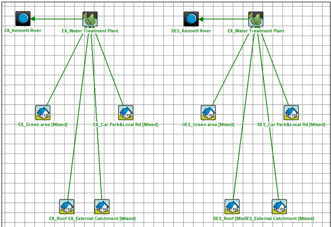
Figure 4-1 MUSIC model layout for the western subcatchment (Ex\_Water Treatment Plant includes sediment pond and wetland)
