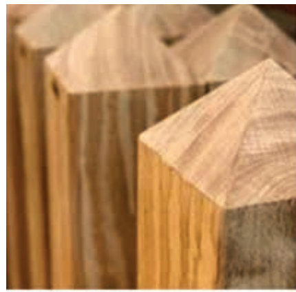
Timber materials used need to be able to oxidise (Silver Off)
