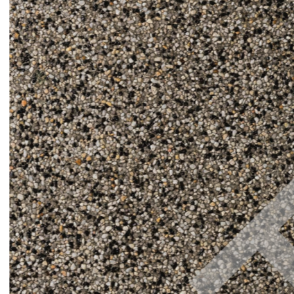
Preferred community exposed aggregate concrete, Point Addis (or similar)
