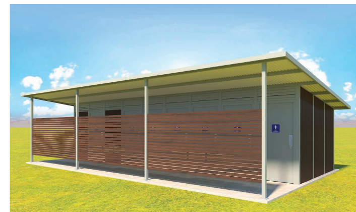
Toilet block with timber battens and steel posts with skillion roof as selected by community. Planting around the toilet block and water tanks used to help blend building into landscape.
