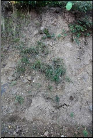
Existing site cut, low strength rock and evidence of colluvium
