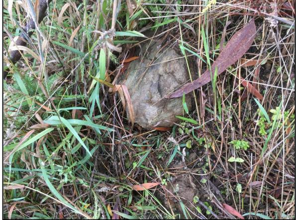
Existing site. Colluvium with embedded cobble/rock, indicating previous landslide movement
