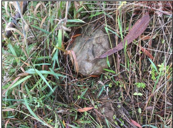
Existing site surface. Colluvium with embedded cobble/rock, indicating previous landslide movement
