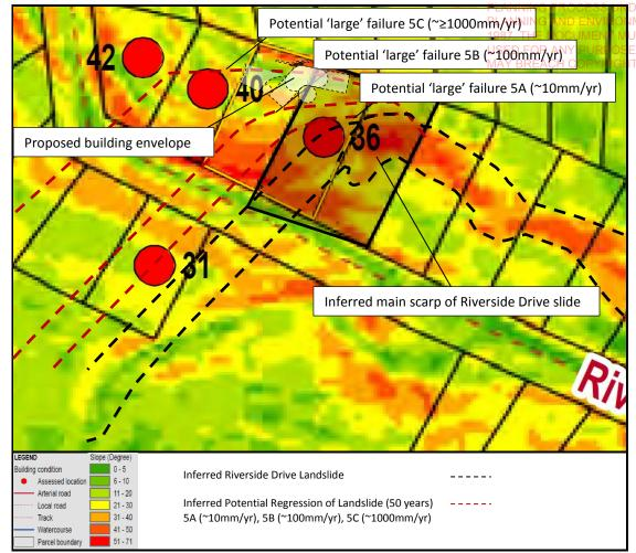
Figure 5: DELWP, Wye River and Separation Creek - Slope Analysis, Coffey 2016
