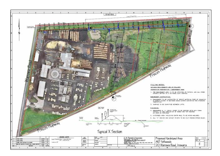
The construction of the proposed earth wall will be located along the north east boundary adjacent to the existing railway line. The total length of the wall proposed is 414 metres, with a maximum height of 3 metres. The earth wall would be off-set approximately 2 metres from the northern boundary and extend into the site for approximately 13.5 metres.
