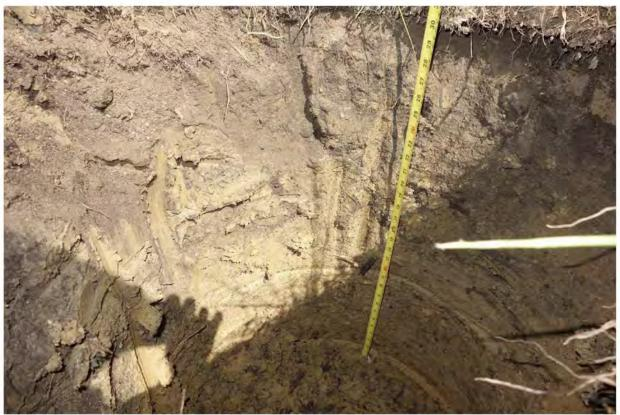
Photo 3 Typical sub-surface conditions at borehole BH3 with Sandy Clay LOAM overlying mottled Medium CLAY at depth.
