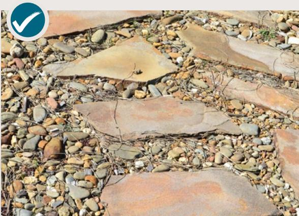
*Non-flammable pathways can be used to separate garden beds to break up fuel continuity.*
