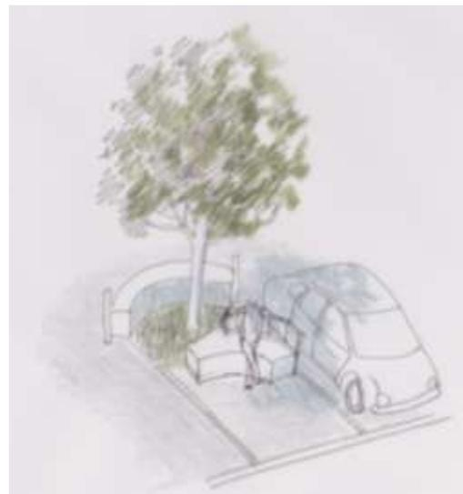
In both instances, fixed installations are set back at least 2.5m from the kerb to allow for mechanical street cleaning.
